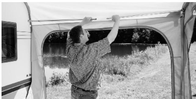
Hang the side roof pole in the threaded fixing eye or Vario Clip on the caravan and connect it to the side bracket. Spread the pole slightly and then tighten the screws completely.
