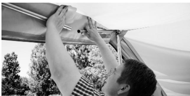
Connect this side bracket with the centre bracket, spread the poles apart slightly and then tighten the screws completely.
